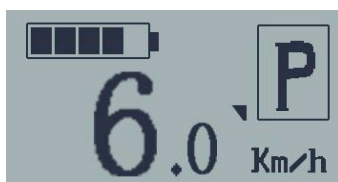
Push-assist display interface
